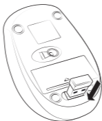
Fig. 6. Fitting the receiver into the mouse case
