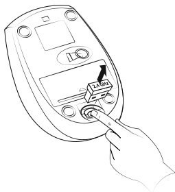
Fig. 5. Extraction of the receiver from the mouse case
