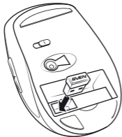
Fig. 6. Fitting the receiver into the mouse case
