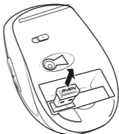
Fig. 7. Extraction of the receiver from the mouse case
