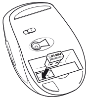
Fig. 6. Fitting the receiver into the mouse case
