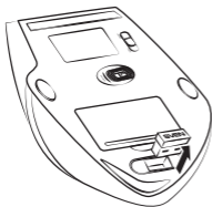
Fig. 5. Extraction of the receiver from the mouse case
