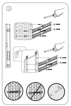
• Fix the wall plate on the wall, as shown in Fig. ③, using suitable accessories from the mounting kit.
