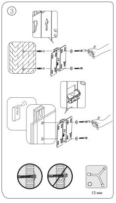
$\bullet$  Fix the mount on the wall using dowels (see Fig. (3)).
