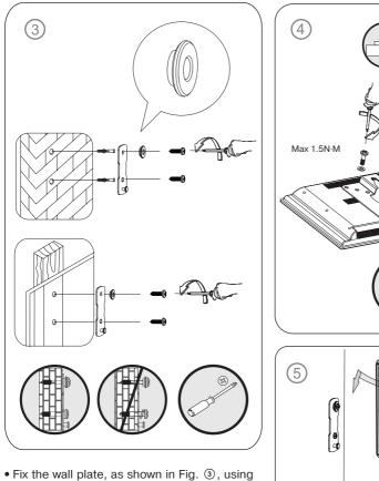
Fix the wall plate, as shown in Fig. (3), using suitable accessories from the mounting kit.
