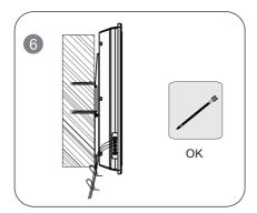
• To unmount your TV, release the security locks (see Fig. ①). Lift your TV slightly and take the mounting system out of the holes.
