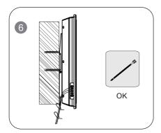
• To unmount your TV, release the security locks (see Fig. ⑦). Lift your TV slightly and take the mounting system out of the holes.
